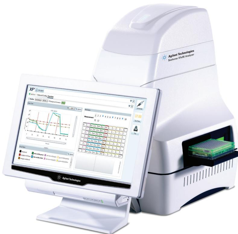
Seahorse XF analyzers are available in 96, 24, and 8-well formats to accommodate a range of throughput and sample needs: adherent and suspension cells, cultured or *ex vivo* samples, model organisms, and isolated mitochondria.
