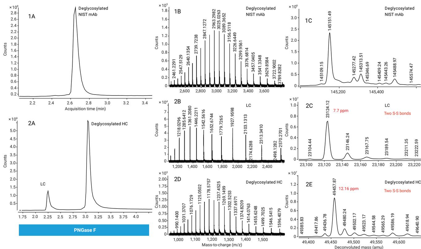
**Figure 10.** 1A, 2A) TIC of Protein L purified intact and reduced NISTmAb after on-cartridge deglycosylation with PNGase F. 1B, 2B, 2D) Mass spectra of deglycosylated NISTmAb, LC and HC. 1C, 2C, 2E) Deconvoluted spectra of deglycosylated NISTmAb, LC and HC. LC = light chain; HC = heavy chain.
