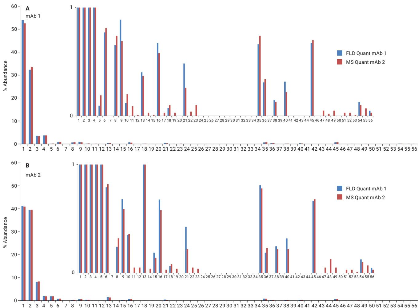
**Figure 8.** Comparison of fluorescence and relative MS abundance (area sum percentage) of InstantPC-labeled N-glycans from mAb 1 and mAb 2. The X-axis represents individual glycan compositions quantified in the study.
