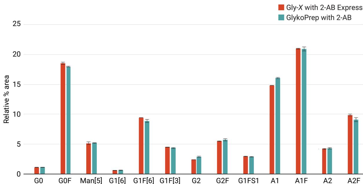
**Figure 8.** Samples produced using the AdvanceBio Gly-X 2-AB Express kit produce data equivalent to samples prepared using older methods, such as ProZyme GlykoPrep 2-AB, shown here for N-glycans from Enbrel. n = 3 for all data.
