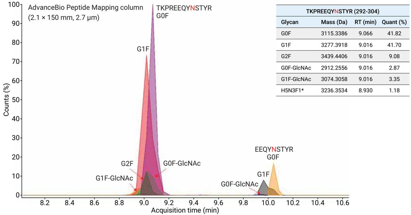
**Figure 6.** MS extracted compound chromatograms (ECCs) and relative % quantitation of the identified glycopeptides from RP LC separation. H5N3F1\* may be denoted as FM4A1G1 or FA1G1Ga1 in other publications.
