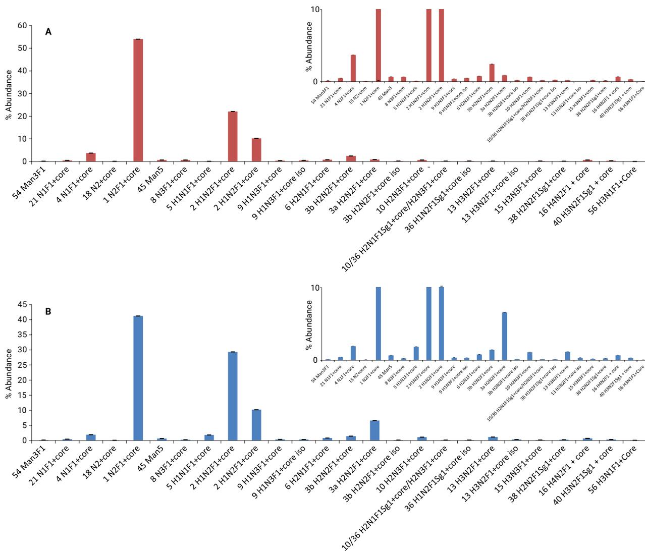
**Figure 4.** A) Relative FLD quantification of mAb 1 glycans. B) Relative FLD quantification of mAb 2 glycans. Error bars represent  $\pm$  standard deviation of quadruplicates having gone through the entire workflow. Integration of FLD signals was performed using Agilent MassHunter Qualitative Analysis Software. Insets show the same data zoomed to better display components with <10 % relative abundance.
