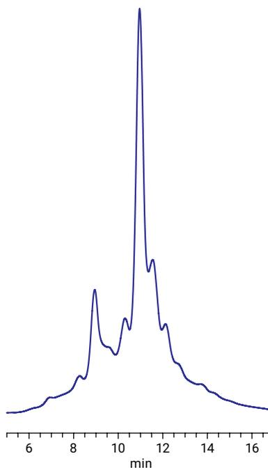
Separation of protein standards on Agilent 3 µm ion-exchange columns by cation-exchange chromatography
