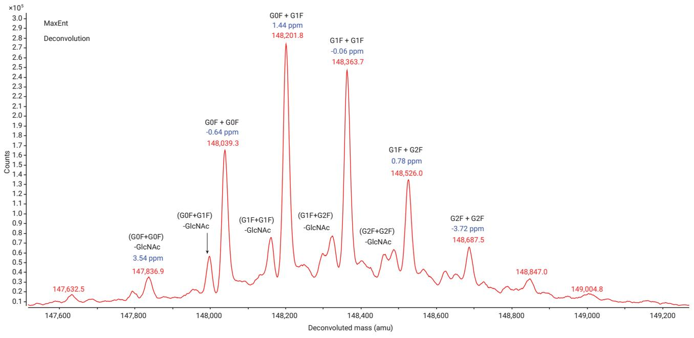
Figure 3. MS Deconvolution of intact NISTmAb (0.5  $\mu$ g injection).
