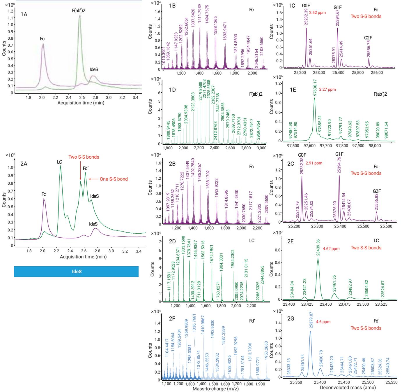
**Figure 8.** 1A and 2A) TIC of subunits from ECD-purified Herceptin after on-cartridge IdeS reaction and reduction. 1B, 1D, 2B, 2D, and 2F) Mass spectra of Herceptin subunits. 1C, 1E, 2C, 2E, and 2G) Deconvoluted spectra of Herceptin subunits.
