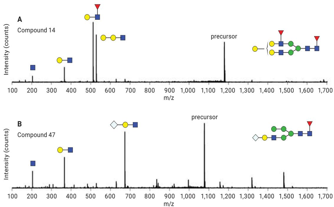
**Figure 6.** Tandem MS data were acquired for all glycans. MS/MS aided in compound identification when accurate mass was insufficient. The two examples above are consistent with gal-gal and outer arm fucose (A) and NeuGC (B) modifications.
