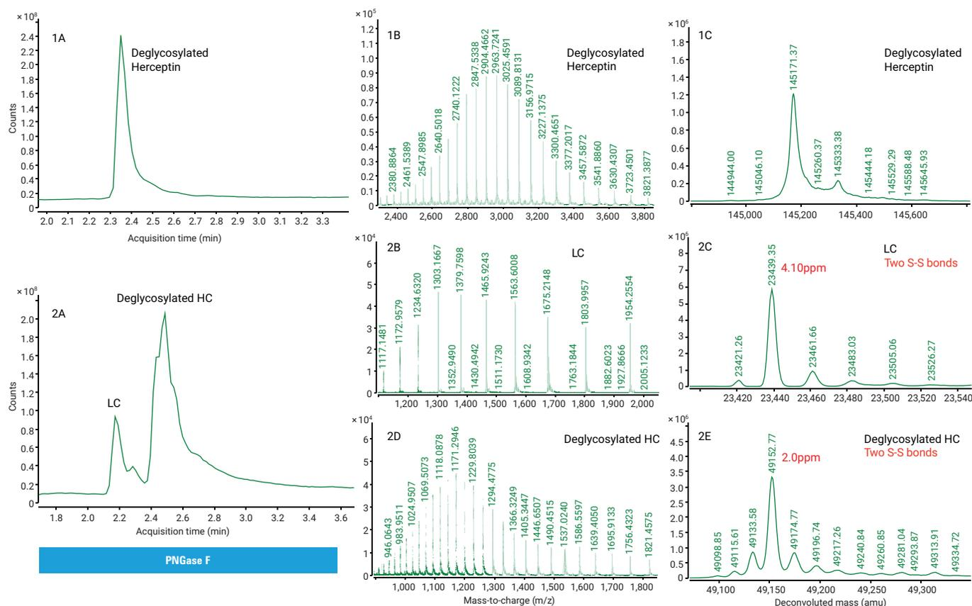
**Figure 7.** 1A and 2A) TIC of ECD purified intact and reduced Herceptin after on-cartridge deglycosylation with PNGase F. 1B, 2B, and 2D) Mass spectra of deglycosylated Herceptin, LC and HC. 1C, 2C, and 2E) Deconvoluted spectra of deglycosylated Herceptin, LC and HC. LC = light chain, HC = heavy chain.
