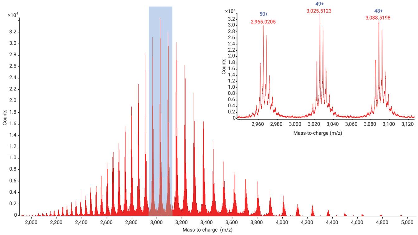
Figure 2. Intact NISTmAb analysis (0.5  $\mu$ g injection).
