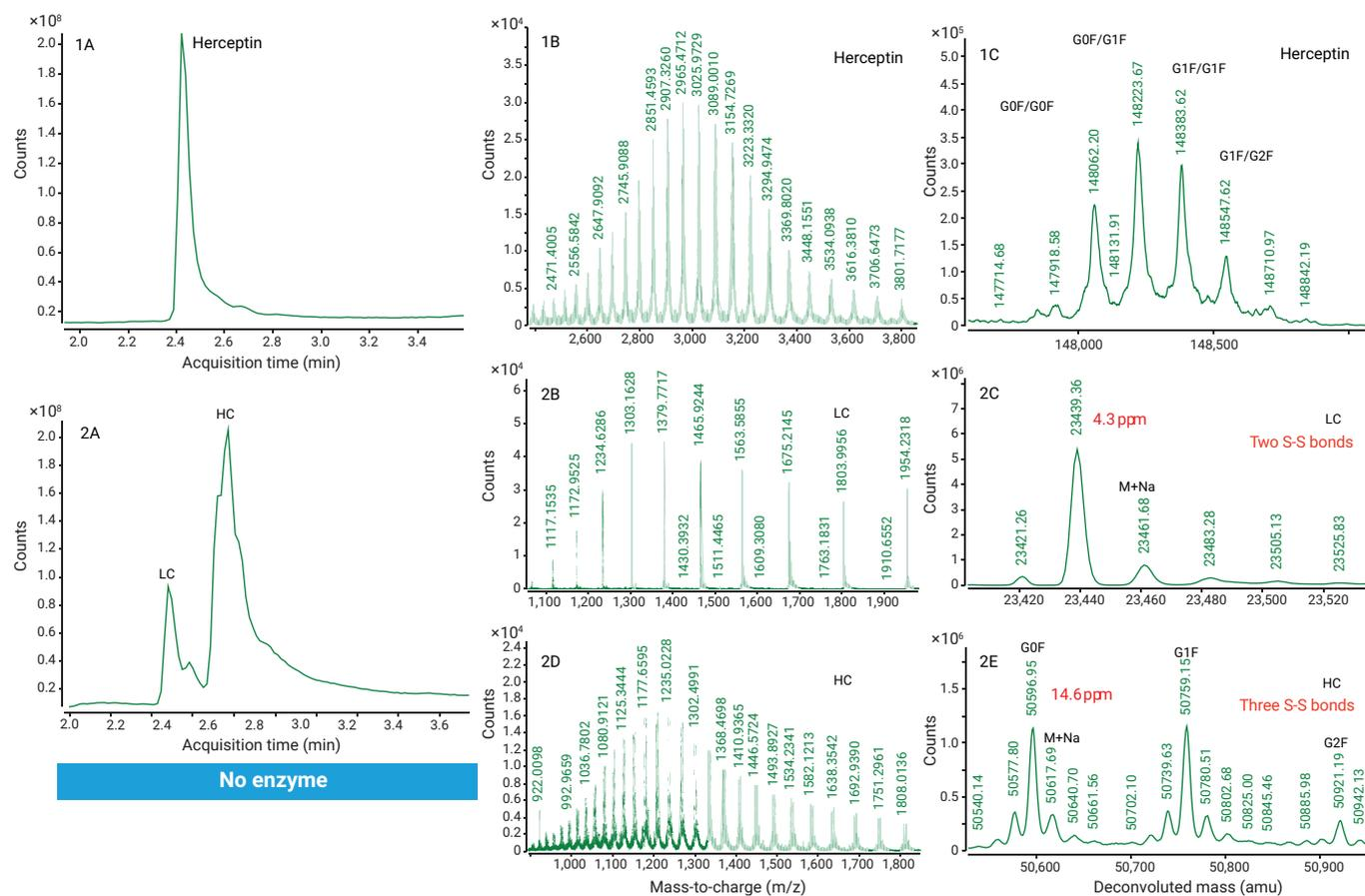
**Figure 6.** 1A and 2A) TIC of ECD purified intact and reduced Herceptin. 1B, 2B, and 2D) Mass spectra of intact and reduced Herceptin. 1C, 2C, and 2E) Deconvoluted spectra of intact and reduced Herceptin. LC = light chain, HC = heavy chain.
