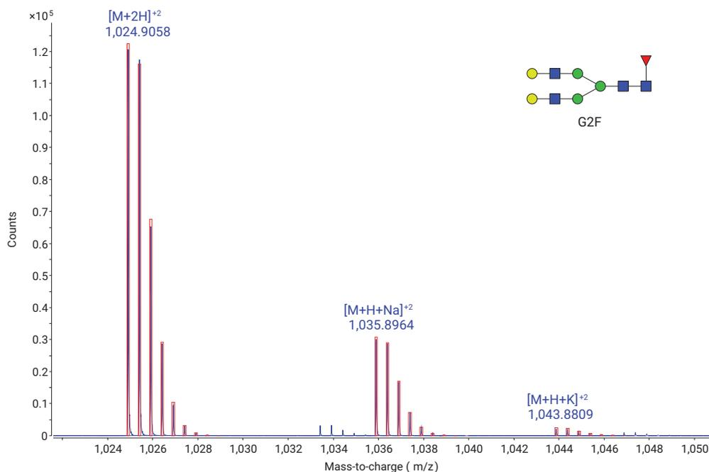
**Figure 4.** Representative spectrum of an InstantPC-labeled N-glycan (G2F). Excellent isotopic fidelity of the charge states of the InstantPC-labeled G2F glycan and its adducts. The red boxes represent the theoretical isotopic pattern, and the blue lines represent the actual raw MS spectrum.
