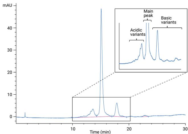
**Figure 1.** Elution profile of pH based separation of charge variants of IgG1 on an Agilent Bio MAb PEEK, 4.6  $\times$  250 mm, 5- $\mu\text{m}$  column. The acidic, main peak and basic variants are enlarged in the magnified view.
