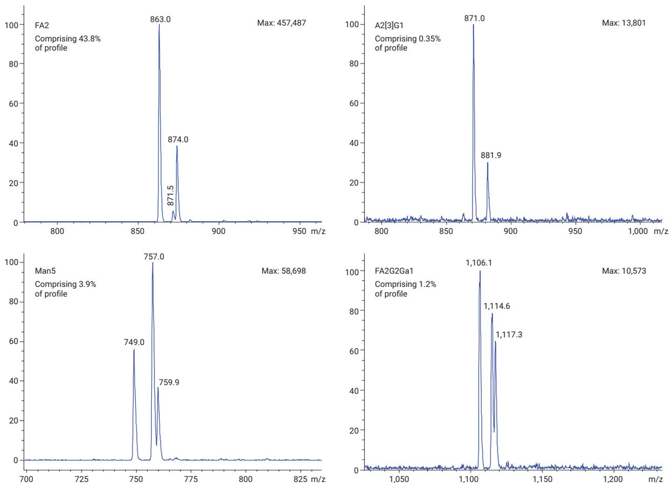
**Figure 4.** Mass spectra of four representative glycans from 3 µg of mAb at various levels of relative abundance. The signal for A2[3]G1, which makes up just 0.35 % of the glycan profile, is clearly observable with a high signal-to-noise ratio.
