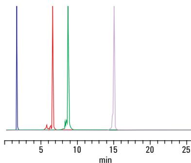
Analysis of a IgG monoclonal antibody using a pH gradient of 6.5 to 7.5 (0-20 min), 50 mM, Agilent Bio MAb, 4.6 x 50 mm, 5 µm
