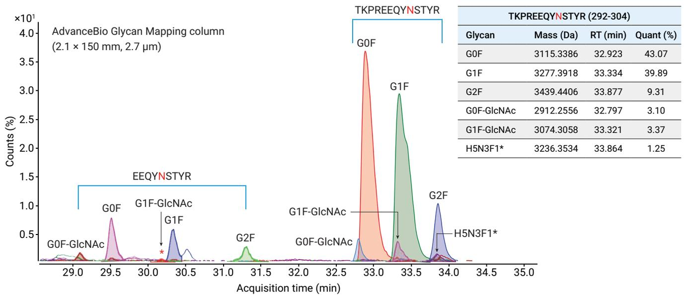
**Figure 7.** MS ECCs and relative % quantitation of the identified glycopeptides from HILIC separation.
