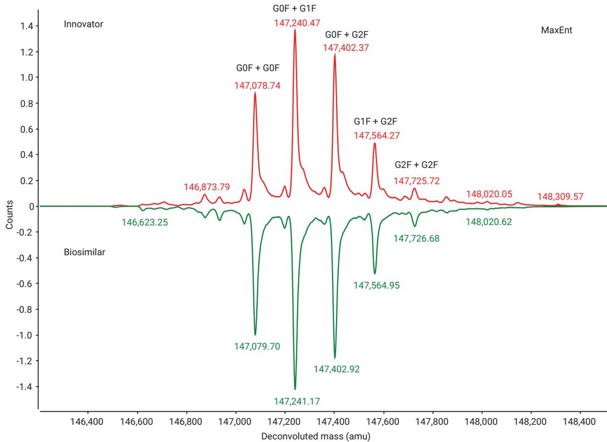
Figure 5. Intact Rituximab analysis (Innovator versus Biosimilar) (0.5 µg).
