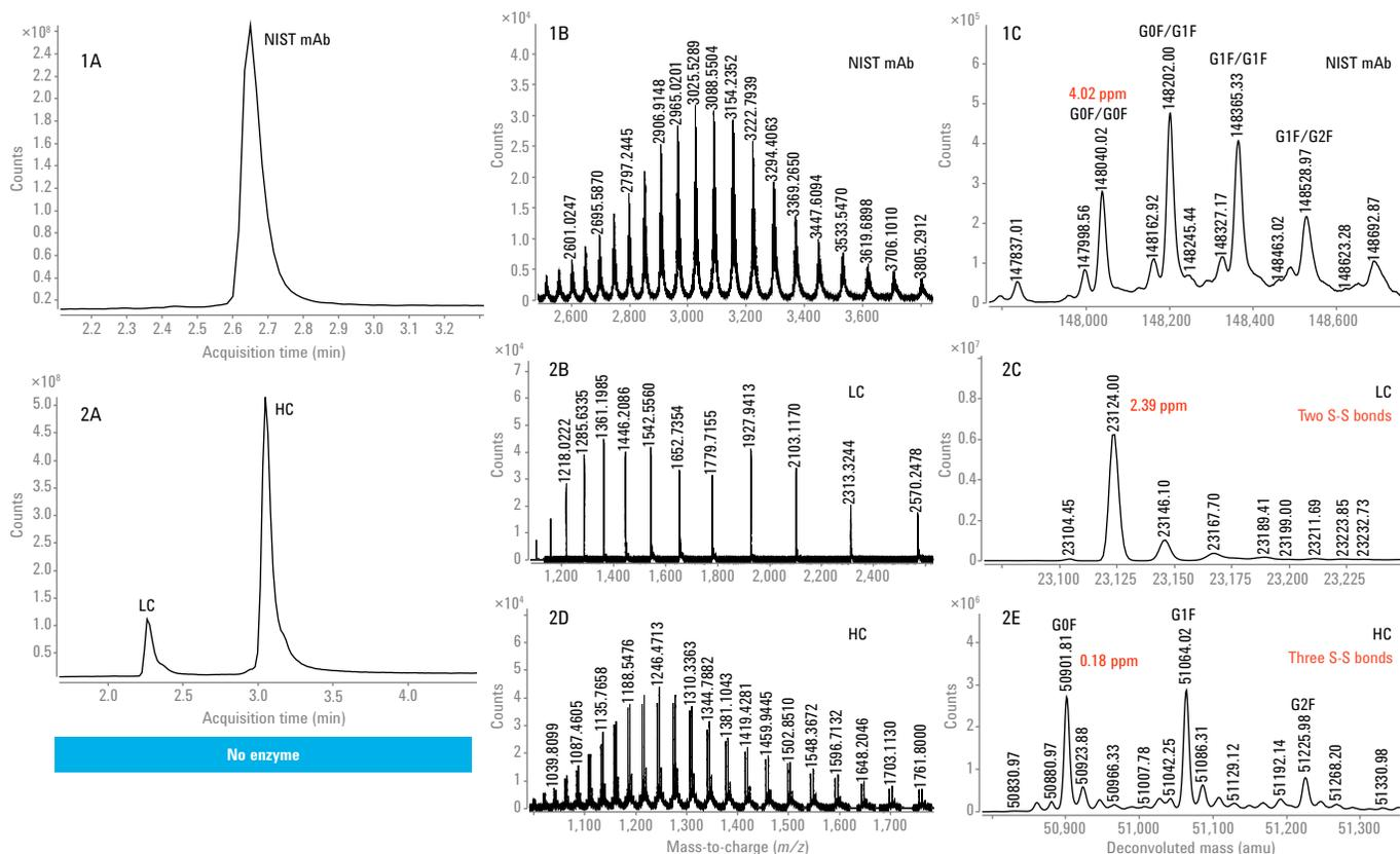
**Figure 9.** 1A, 2A) TIC of Protein L purified intact and reduced NISTmAb. 1B, 2B, 2D) Mass spectra of intact and reduced NISTmAb. 1C, 2C, 2E) Deconvoluted spectra of intact and reduced NISTmAb. LC = light chain; HC = heavy chain.
