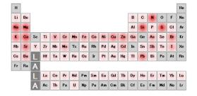
Spot unexpected major elements, unusual levels of analytes, and sample preparation mistakes just by looking at the heat map periodic table produced by the IntelliQuant function.
