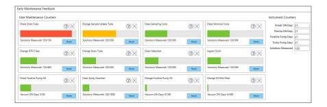
The 7850 uses early maintenance feedback (EMF) sensors and counters to determine when maintenance is needed, based on operation time or number of samples measured. The traffic light color-coded alerts indicate when maintenance tasks are required.
