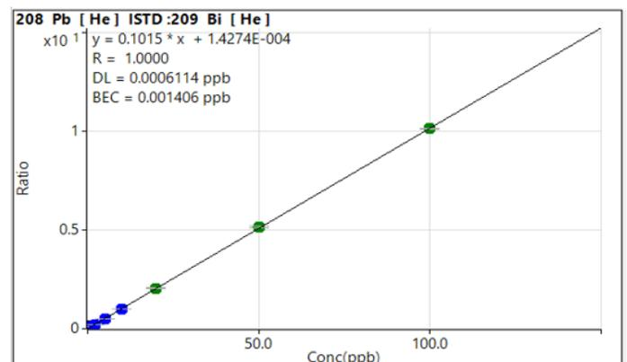
**Figure 2.** Representative ICP-MS calibration curves for Be, As, Cd, and Pb that were automatically created from a single stock solution by the Agilent ADS 2 fitted to the Agilent 7900 ICP-MS.
