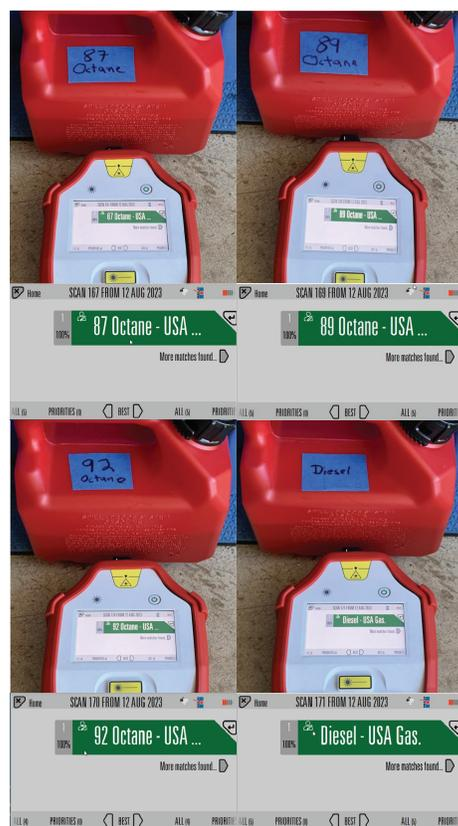
**Figure 6.** 100% match values for the four fuel sample measurements conducted through thick, red plastic containers using the Agilent Resolve and the custom "Fuels" library.
