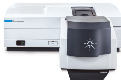
Figure 3. Cary 7000 UMS measures absolute reflectance and transmittance, at almost any angle of incidence, unattended.
