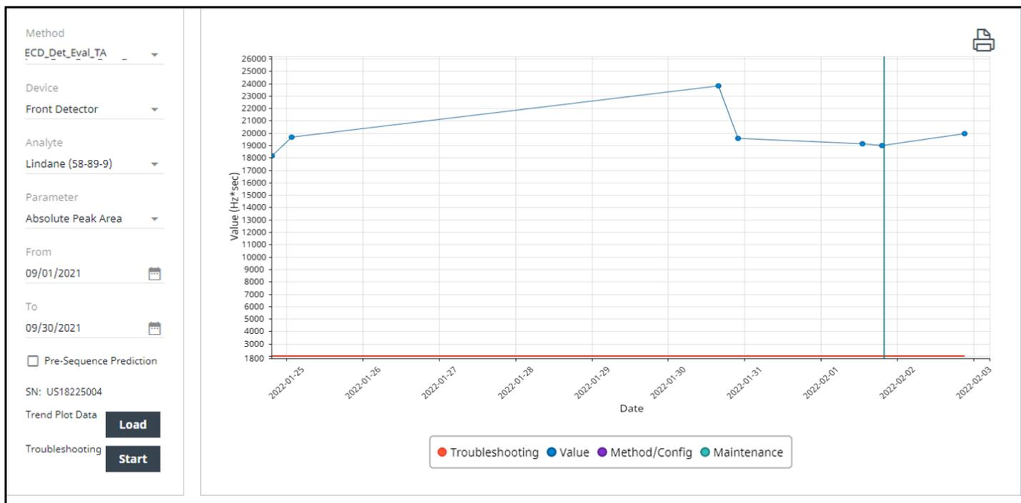
Figure 16. Detector evaluation trend plot example.
