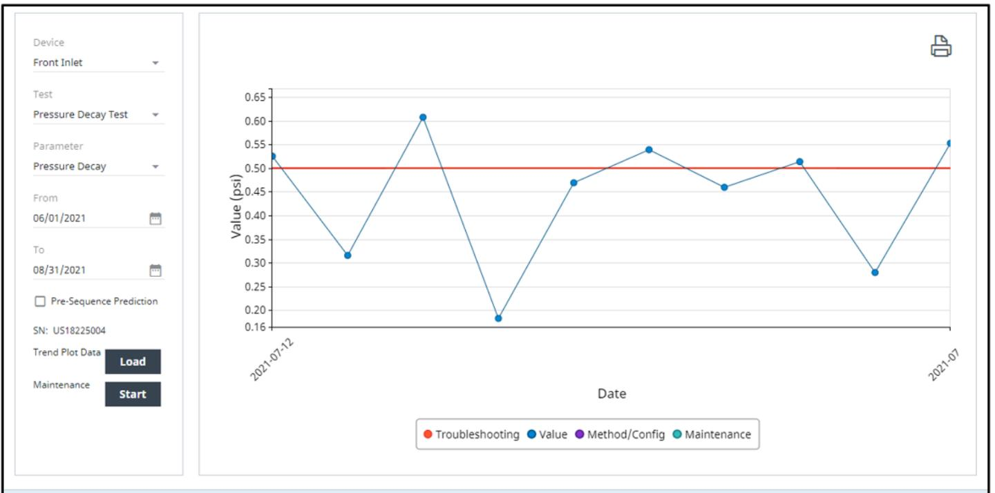
Figure 13. Diagnostic plot of a GC's front inlet pressure decay results.
