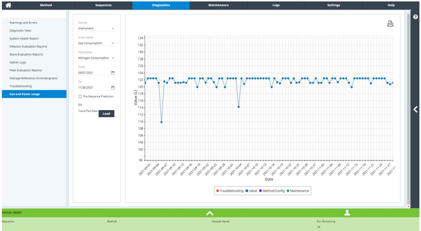
Figure 24. Gas and power use plot showing daily nitrogen consumption over a three-month period.
