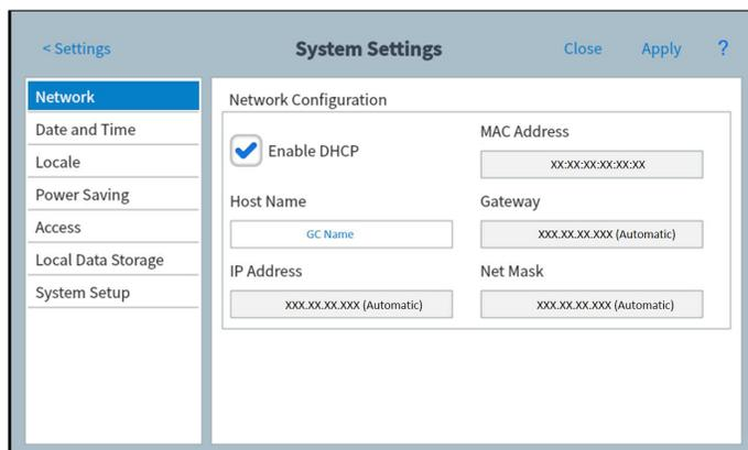
**Figure 1.** Network Configuration window on the Agilent 8890 and 9000 GC touch screen. Navigation path: Settings > System Settings > Network.
