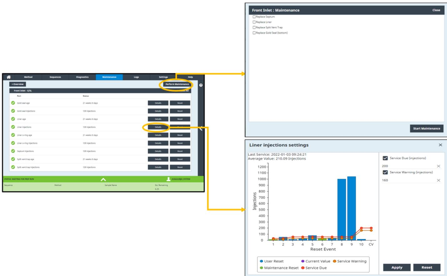
**Figure 26.** From within a specific component, the user can choose a guided maintenance procedure (top right) or view the past use of a component and enable limits for tracking use (lower right).
