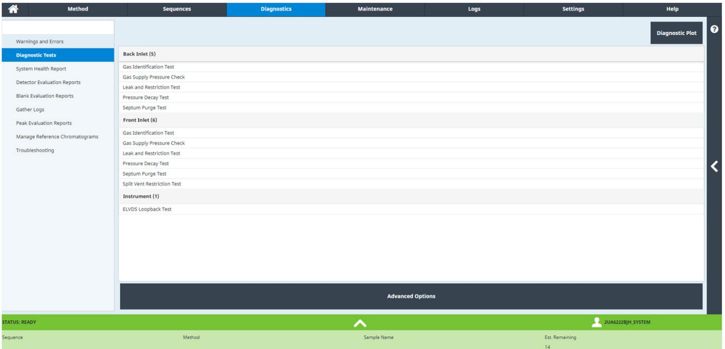
Figure 12. Diagnostic tests available for the HW configured on the GC are listed under Diagnostic Tests in the Diagnostics window.
