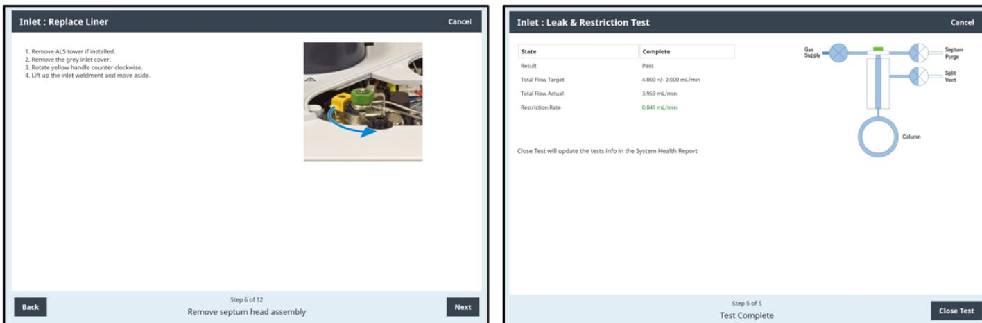
Figure 27. Relevant pictures are used during maintenance procedures to guide users (left) and automated diagnostic tests are used at the completion of a maintenance procedure to verify it was done correctly (right).
