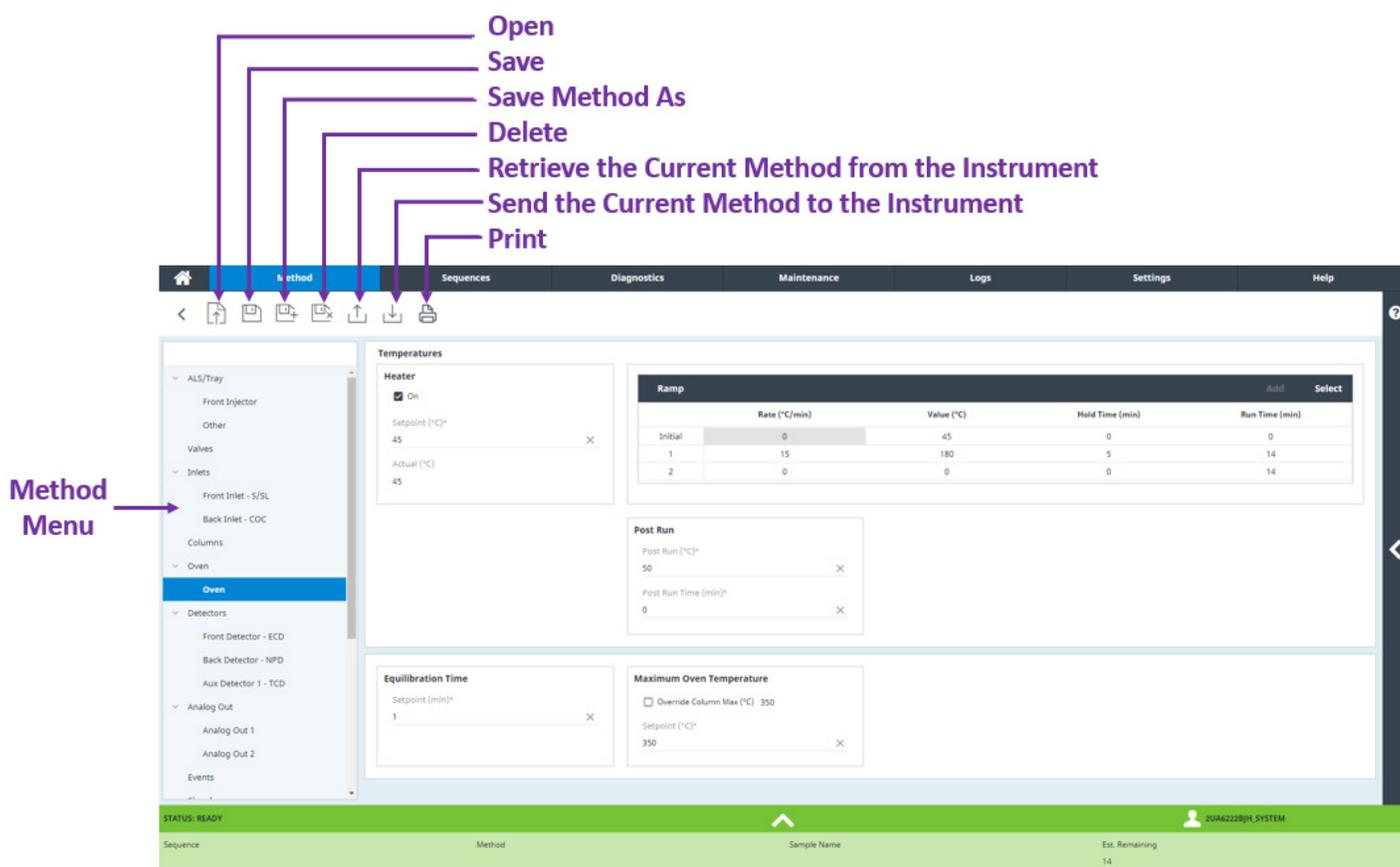
Figure 7. The browser's Method Editor; the layout, iconography, and navigation are consistent with Agilent OpenLab CDS.
