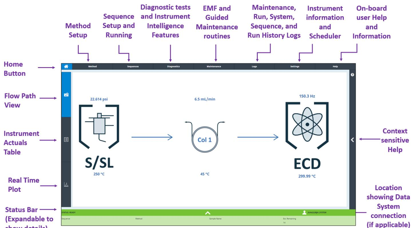
Figure 3. Browser home screen and menu tab identification; flow path view tab shown.
