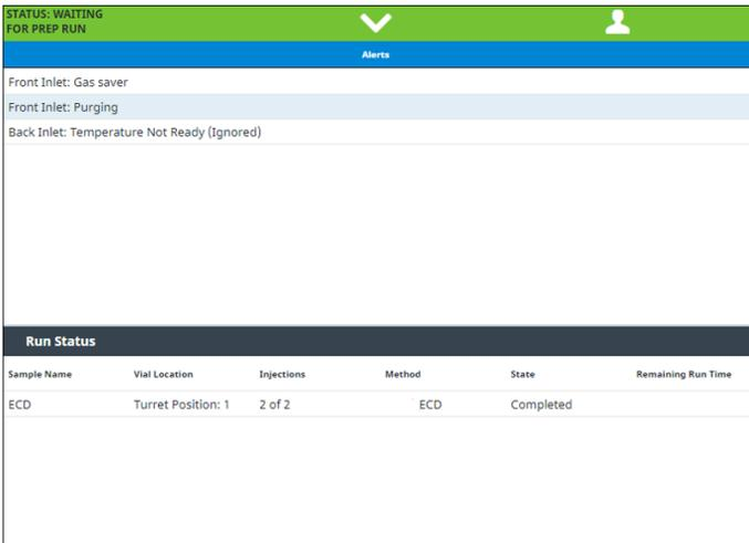
Figure 4. Detailed status information found in the expanded status bar.
