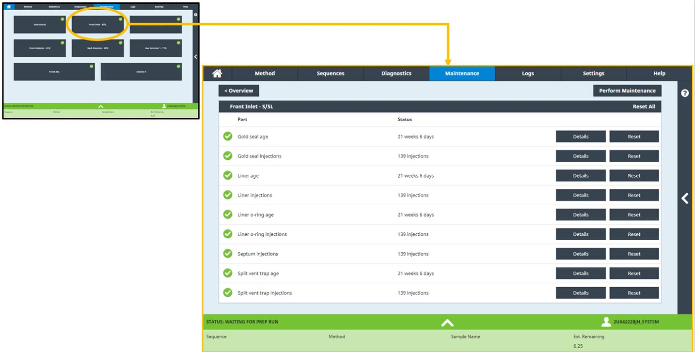
Figure 25. Maintenance tab of the browser interface showing the Front Inlet - S/SL window.
