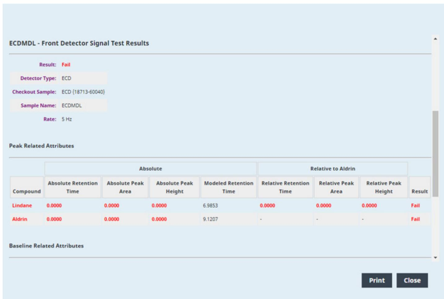
Figure 15. Detector Evaluation Report: an example report for a failed detector evaluation is shown.
