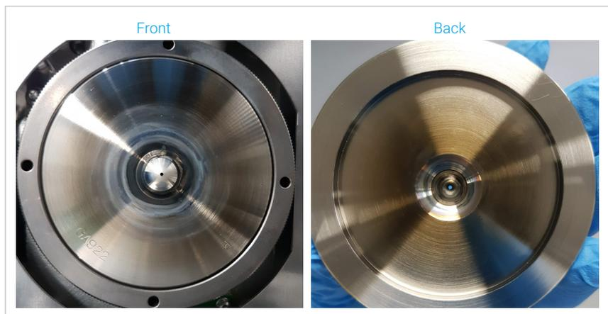
Our new nickel-plated platinum-tipped sampler cone shows almost no copper corrosion (front and back) after 1,090 hours of run time with a 10% aqua regia matrix.
