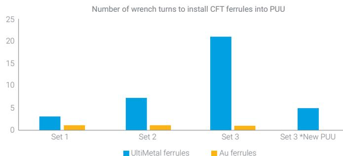
\*Column broke after 20 additional small wrench turns and therefore a new purged ultimate union (PUU) had to be installed.
